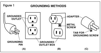
3. The temporary adapter should be used only until a properly grounded outlet (sketch A) can be installed by a qualified electrician. The green colored rigid ear, lug or the like extending from the adapter must be connected to a permanent ground, such as a properly grounded outlet box cover. Whenever the adapter is used, it must be held in place by a metal screw. (See Figure 1)
