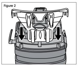
Press down until tabs snap into place. Remove tank cover from tank and refer to the set up and operation section. (See Figure 3)
